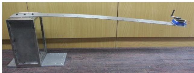
Fig. 3. A wireless accelerometer on a cantilever beam
