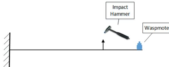
Fig. 2. Test setup and the data acquisition point
