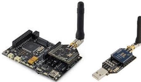
Fig. 1. Wasp mote with ZigBee and the host gateway
