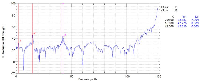
**Fig. 5.** Frequency response function using wireless MEMS accelerometer
