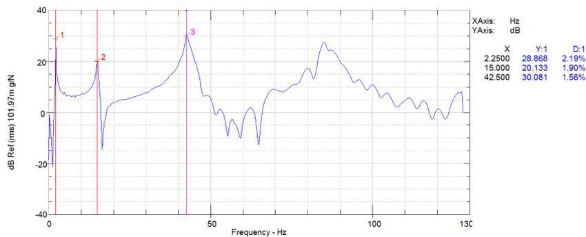
**Fig. 4.** Frequency response function using wired IEPE accelerometer
