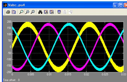
**Fig. 4.** Modulated voltage waveform with the carrier signal of 290 kHz and 300 mA
