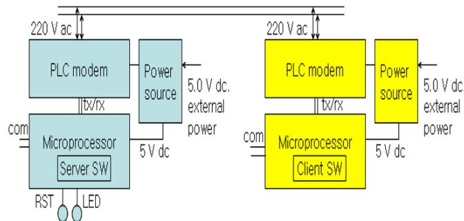
**Fig. 3.** Architecture of proposed cable identification systems
