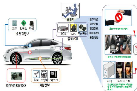
Fig. 1. Schematic diagram of drunk driving ignition interlock system
