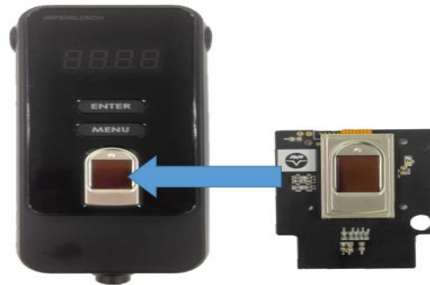
Fig. 2. Alcohol measuring instrument integrated with fingerprint recognition sensor
