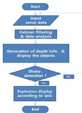
**Fig. 1.** Flow chart of proposed algorithm
