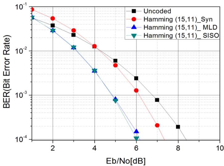
Fig. 2. Bit error rate performance for (15,11) Hamming code
