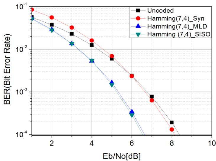
Fig. 1. Bit error rate performance for (7,4) Hamming code
