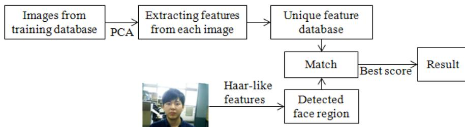
**Fig 2:** The workflow of face recognition subsystem
