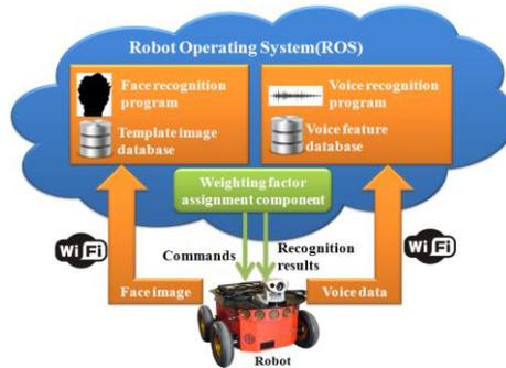
**Fig. 1:** Architecture of multimodal biometric recognition system
