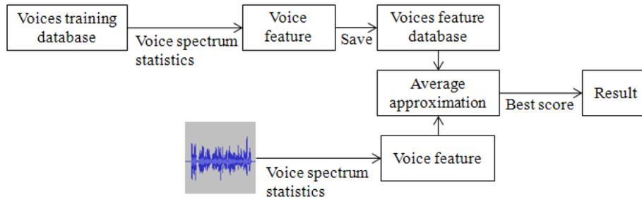
**Fig. 3:** The workflow of voice recognition subsystem
