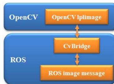
Fig. 3. Communication model between OpenCV and ROS
