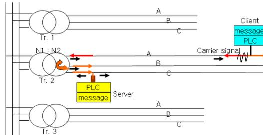
**Fig. 2.** Flow of operation to identify transformers.
