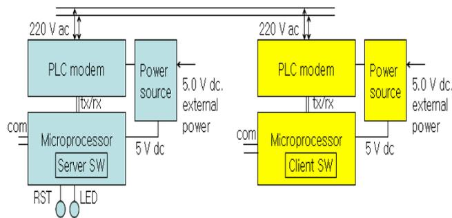
**Fig. 4** Architecture for cable identification system
