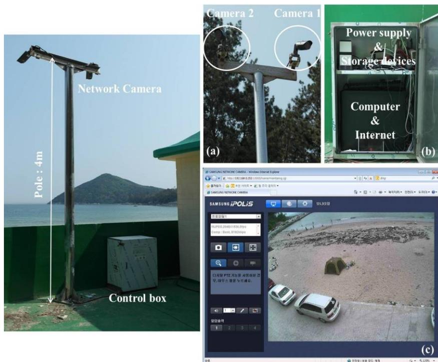
**Fig. 2.** The structure of the network camera system: (a) a network camera setting on a 4-m-high pole (SNO-7080R), (b) the structure of the control box, and (c) the web browser for real-time monitoring.
