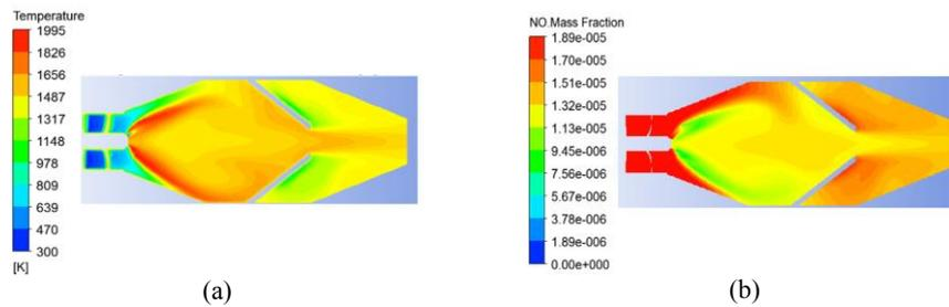
Fig. 2. Flow visualization in can-combustor (a) Temperature contour & (b)  $\text{NO}_x$  mass fraction
