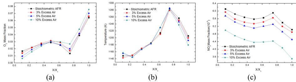
**Fig. 3.** Graphical representation of the flow in can-combustor (a)  $\text{O}_2$  mass fraction, (b) Temperature magnitude & (c)  $\text{NO}_x$  mass fraction of the combustor along the center line for different AFR
