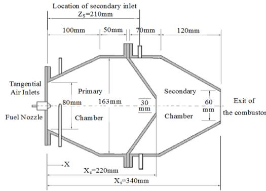
Fig. 1. Schematic diagram of the can combustor model
