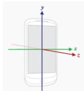
Fig. 1. Sensor Coordinate System
