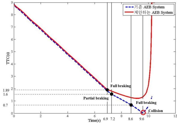
Fig. 2. TTC changes at road and speed conditions (snow asphalt:  $\mu = 0.3$ ;  $v$ : 40 [km/h]).
