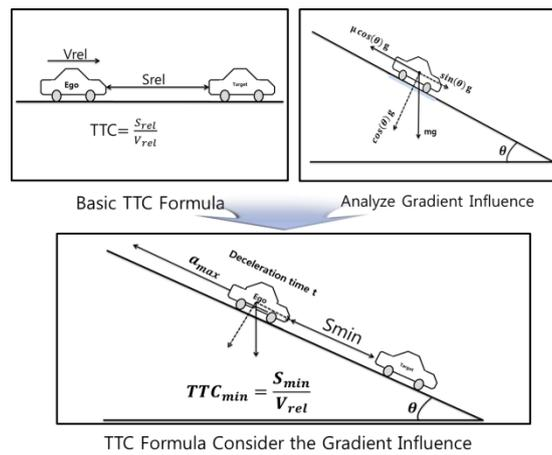
Fig. 1. Block diagram of TTC calculation method that considers a gradient.
