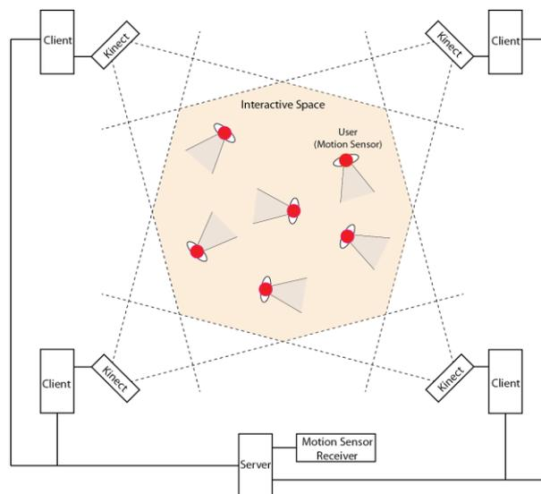
Fig 2. Body tracking system for multiple users
