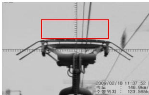
Fig. 2. Pantograph and Region of Interest (ROI)
