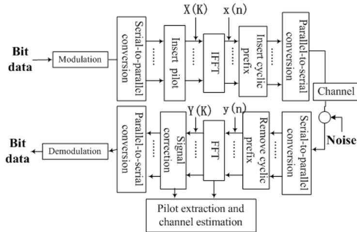
Fig. 1. Transmission diagram of Pilot method of OFDM system
