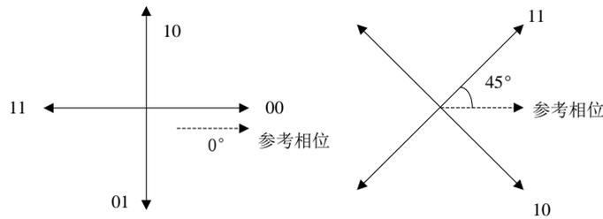
**Fig. 2.** QPSK modulation vector diagram.
