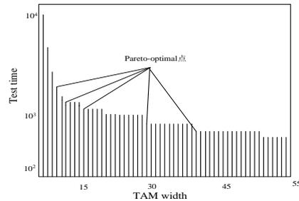
Fig. 2. TAM width and test time relationship
