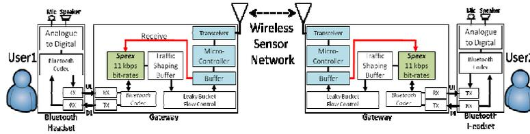
Fig. 2 BZVG system architecture
