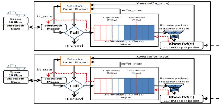
Fig. 3 Architecture of BZVG flow control
