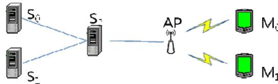
Fig. 2. The network topology of the simulations
