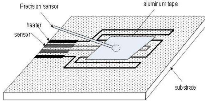
**Fig. 2.** Precision sensor attached to the biochip surface.
