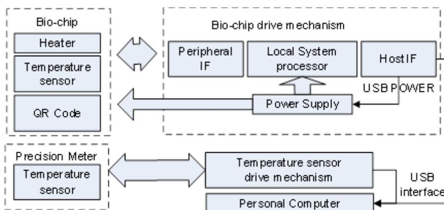
Fig. 1. Block diagram of biochip calibration system and QR code recognition system.
