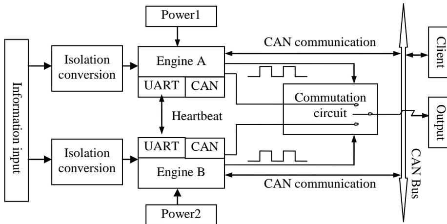
Fig. 1 Controller structure based on warm standby
