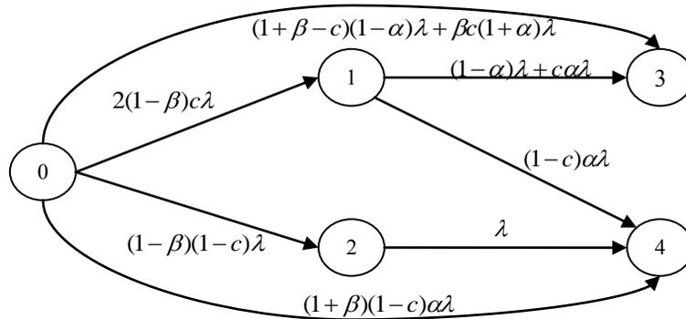
Fig. 2 State transition diagram of dual computer hot stand-by system
