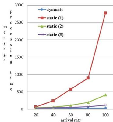
Fig. 2. Message processing time as to implementation structure of threads
