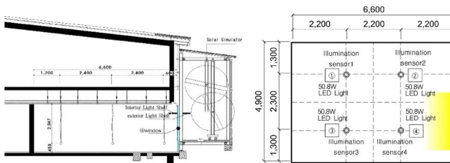
Fig. 1. View of Test Bed and Position of the illuminance sensor Ceiling
