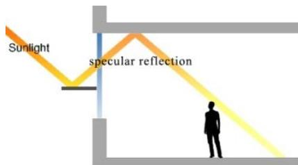
Fig. 2. The principle of the shelf system of light[1]
