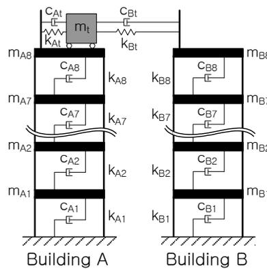
**Fig. 1.** Configuration of STMD
