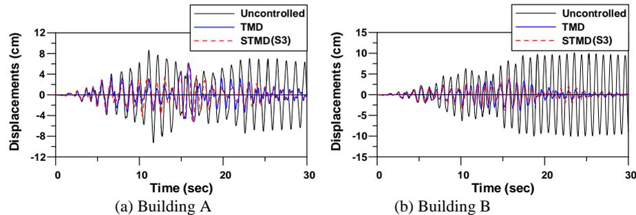
Fig. 2. Top floor displacements of artificial earthquake
