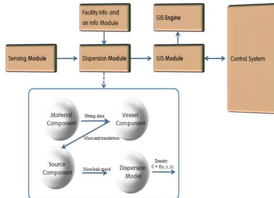
**Fig. 1.** Design of real-time atmospheric dispersion system
