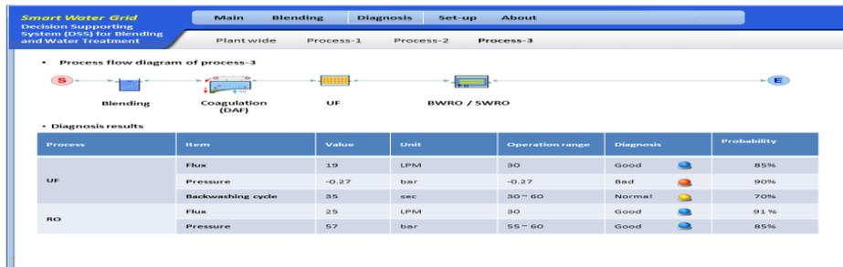
Fig. 4. Process diagnosis with seawater and brackish water for WTP
