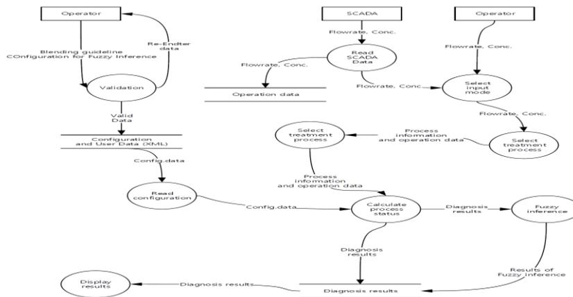
Fig.2. Data Flow Diagram of process diagnosis for WTP
