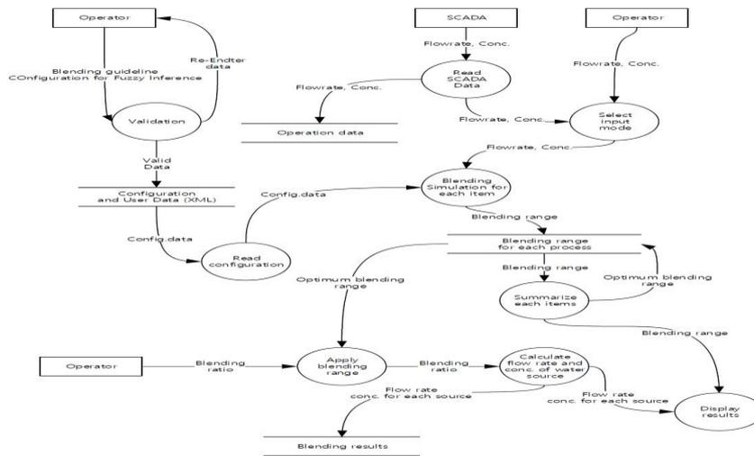
Fig. 1. Data Flow Diagram of process operation for optimum blending value of WTP
