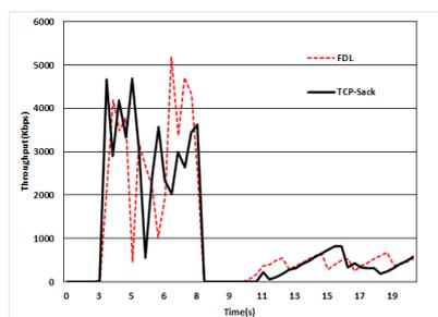
**Fig. 6.** Throughput in Upward handover when errors are occurred
