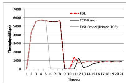
**Fig. 5.** Throughput in Upward Vertical Handover
