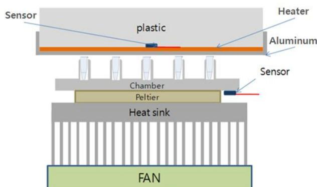
Fig. 1. Configuration of hardware components
