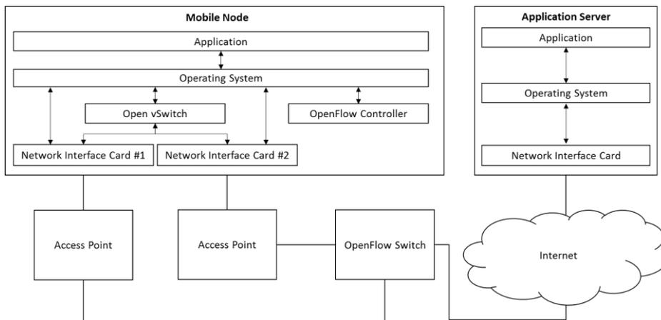
Fig. 1. Proposed mobile network and device structure
