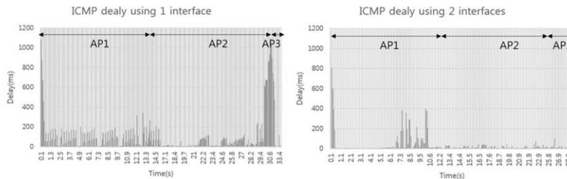
**Fig. 2.** (a) ICMP delay of mobile node using single interface. (b) ICMP delay of mobile node using dual interface
