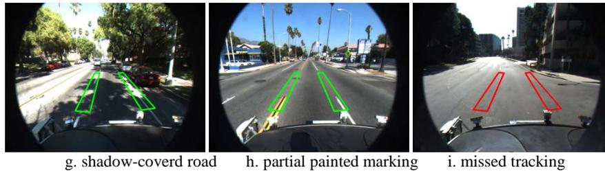
**Fig.3.** Lane marking detection results
