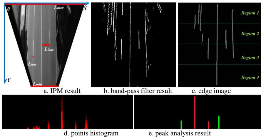
**Fig.2.** Lane marking detection
