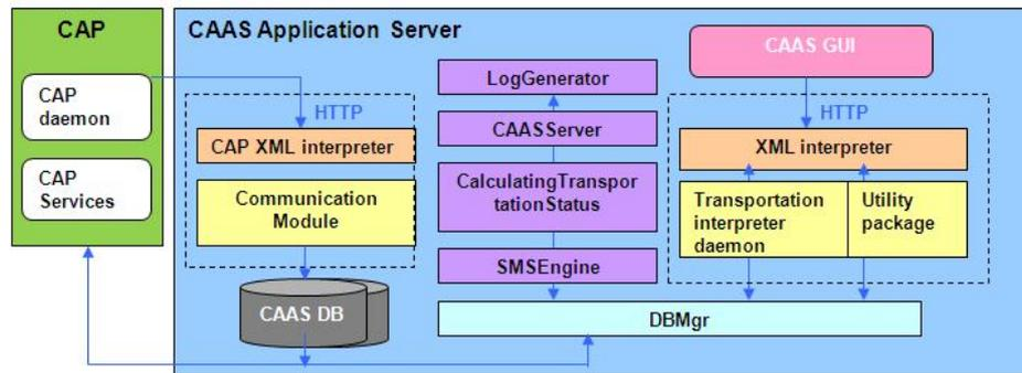
Fig. 1. The Core CAAS Main Functions
