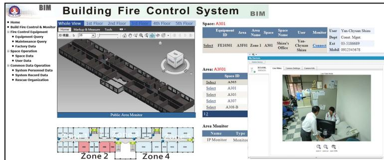
Fig. 1. Building fire control display and monitor video display
