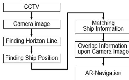
Fig. 1. Process of computer image processing to build AR-based sea navigation scene.
