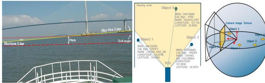
Fig. 5. Horizon line and calculate pose (left) and area filter by using AIS and GPS data (right)
