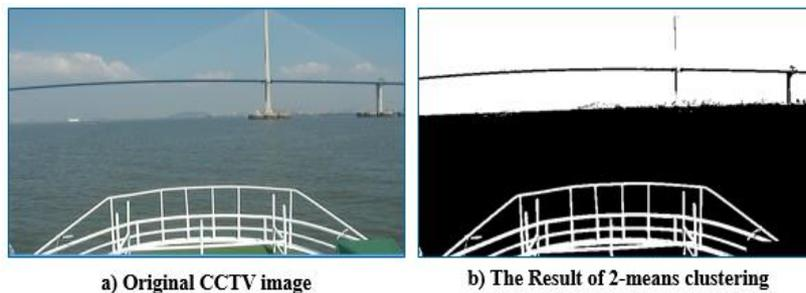
**Fig. 3.** Original CCTV image (left) and 2-means clustering result (right): 2-means clustering can divide the image into sky side and the other side well.
