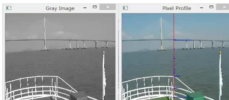
**Fig. 2.** Gray scale image (left) and result of pixel profiling (right): the pixel profiling and Hough Transform were disturbed by the bridge.
