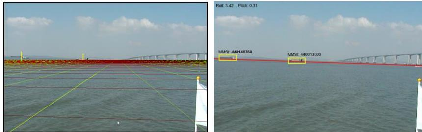
**Fig. 6.** Planar registration upon a sea surface (left) and Result of ship and horizon line detection (right)
