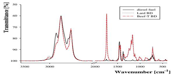
Fig. 3. FTIR spectra of experimental fuels
