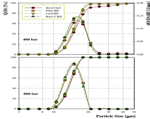
Fig. 2. Droplet size distribution of experimental fuels
