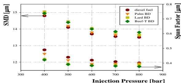
Fig. 1. Variation of SMD and span factor of experimental fuels
