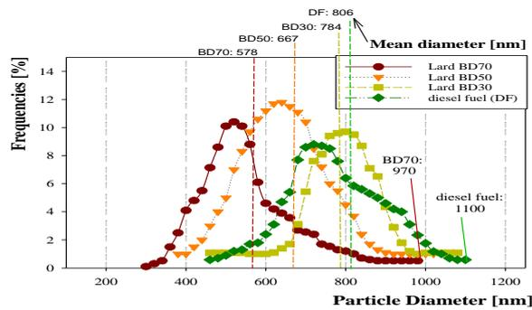
Fig. 4. Particle number and size distribution of experimental fuels
