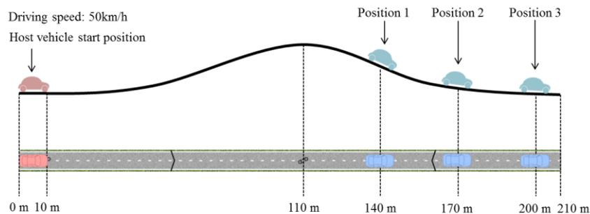
**Fig. 1.** Simulation scenario for performance limits analysis of automotive radar
