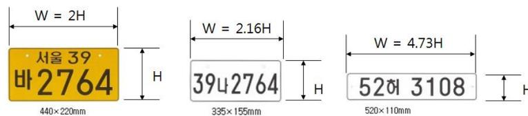
**Fig. 1.** Sizes of car number plates used in Korea
