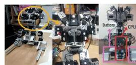
Fig. 12. Cat robot skeleton and motor installation
