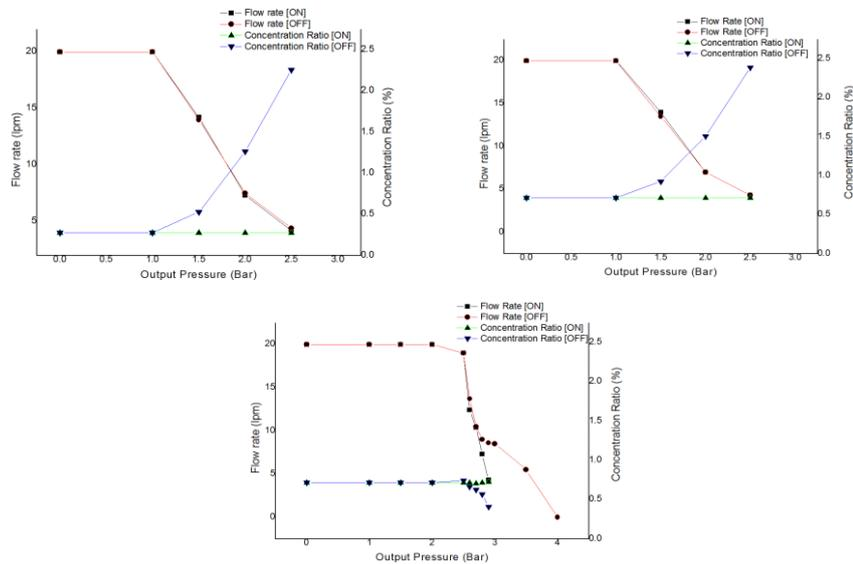
**Fig. 40** Mixed Gas Flow Rate and Its Concentration of the SF6 according to the Outlet Pressure (Case 1, 2, 3)
