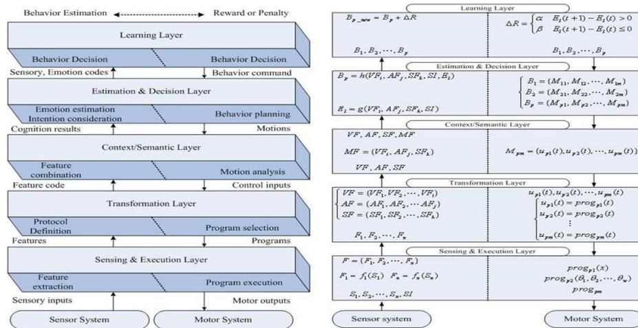
Fig. 3. 5 Layer structure with definition of functions and protocol
