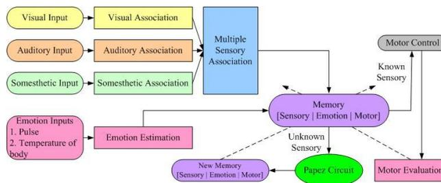
Fig. 2. Block diagram of behavior decision using Papez circuit
