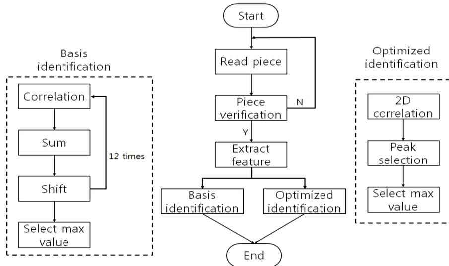
**Fig. 2.** Flowchart of existing and optimizing identification method
