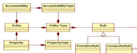
Fig. 5. Depicts the core design of an AOM
