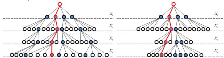
**Fig. 1.** Tree diagram example of the fixed QRD-M( $M=4$ ) and the QRD-S for QPSK modulation with 4 by 4 antenna system.
