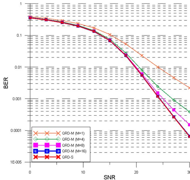
**Fig. 2.** The BER of the conventional QRD-M ( $M=1, 4, 8, 16$ ) and the QRD-S detection scheme with 8 by 8 MIMO-OFDM with 16-QAM system.
