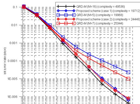
**Fig. 1.** BER performance of the conventional and the proposed detection schemes in the  $8 \times 8$  antenna system.
