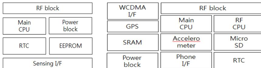
**Fig. 2.** Architecture of sensor tags & base stations.
