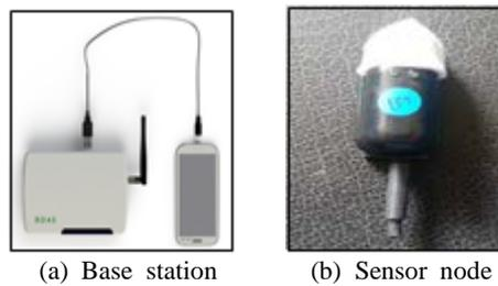
**Fig. 1.** Implemented base station and sensor node
