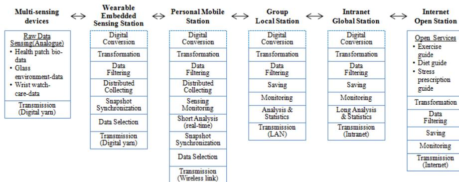
Fig. 2. Multiple sensing bio-information operations.
