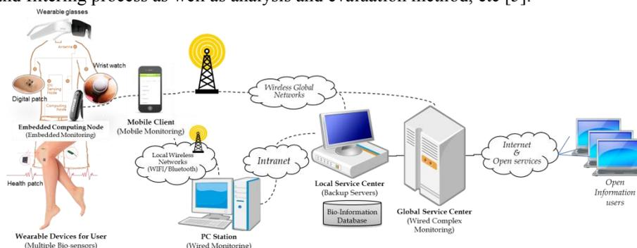
**Fig. 1.** Wearable multiple sensing architecture for bio-information computing.
