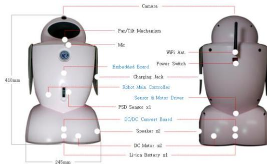
Fig. 2. Appearance and specifications of the service robot.
