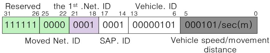
Fig. 2. The format of virtual IP address
