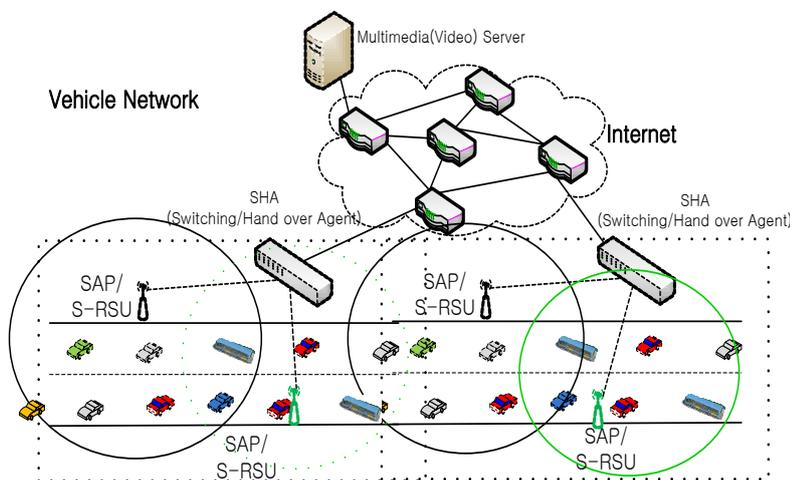
**Fig. 1.** The structure of the proposed seamless multimedia service system in VCN network
