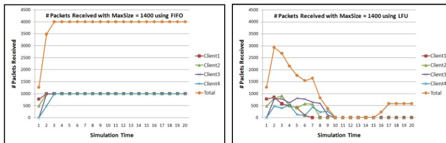
Fig. 3. The number of packets received with 1400 entries with using FIFO and LFU
