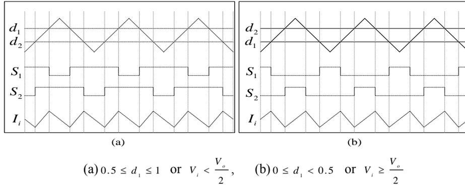
Fig. 3. Key waveform of the proposed three level boost converter
