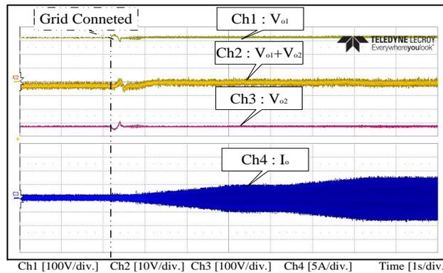
Fig. 5. Waveform of grid-connected experiment
