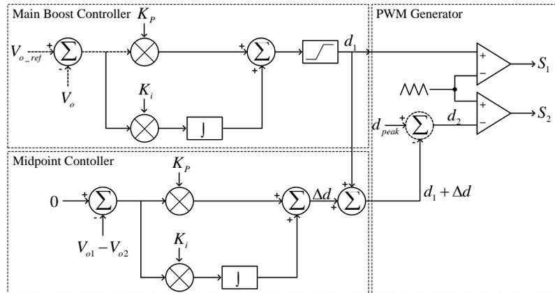
Fig. 2. Block diagram of the purposed boost converter controller
