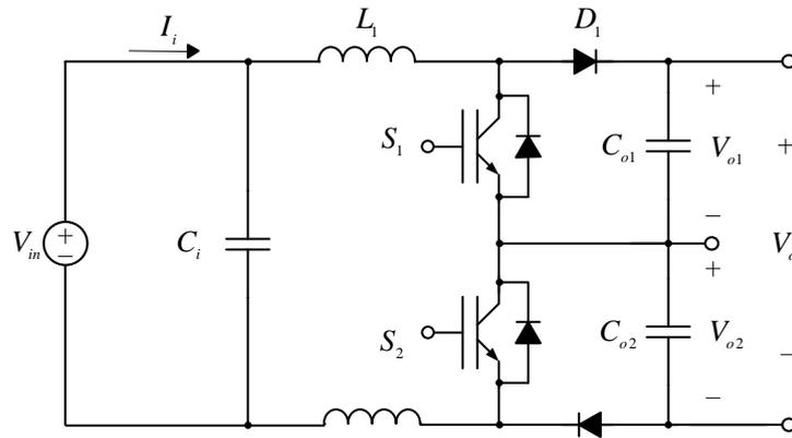
Fig. 1. Schematic of three level boost converter
