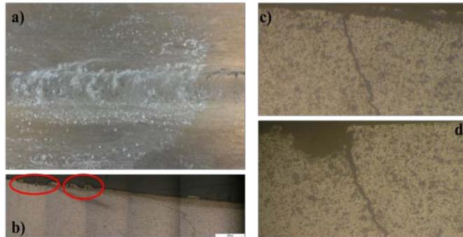
Fig. 2. – Samples submitted to corrosion testing: a) corroded plate, b) Top of the sample, c) sample with defect before corrosion testing and d) sample with defect after corrosion testing
